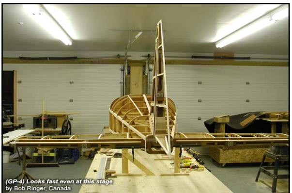
(GP-4) Fin, rudder and stabilizer ready for skin by Bob Ringer, Canada
