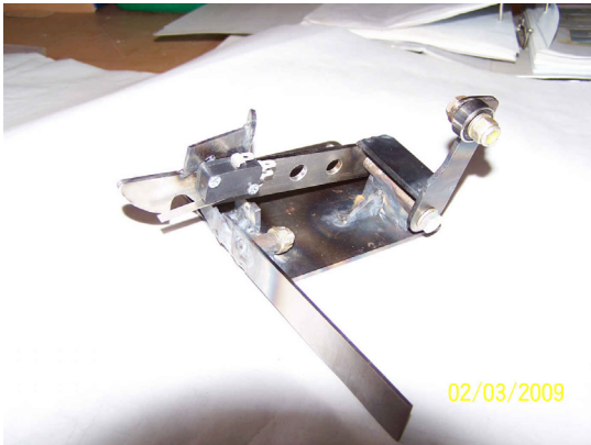
Uplock unit. Note offset of roller arm for release cam. The offset is because of the reversing of ram/retract. arm
