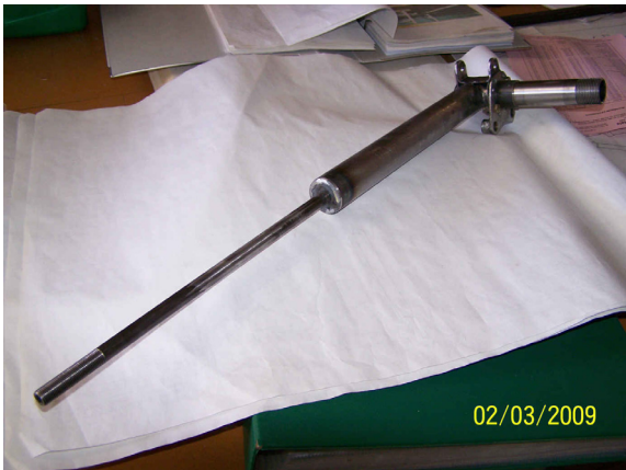
Upper rod, with thread cut...to be trimmed to length when installed in wing.
