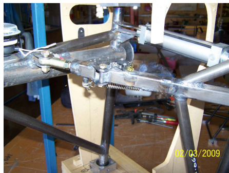
The retract link and ram reversed. Link connected to leg with clevis and rod end bearing.
