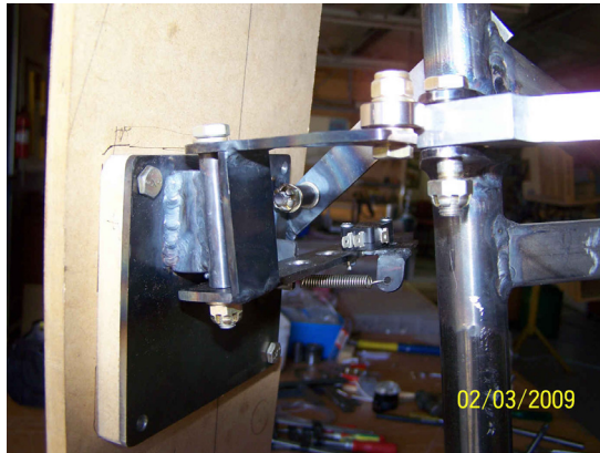
Uplock unit. Note offset of roller arm for release cam. The offset is because of the reversing of ram/retract. arm
