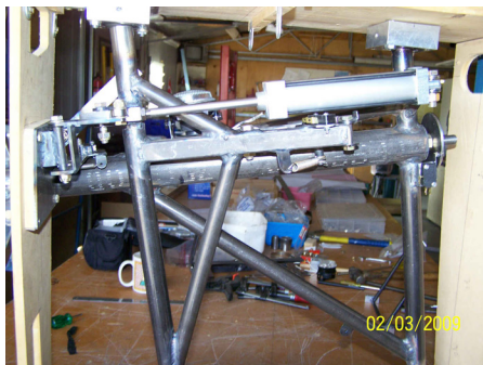
The retract link and ram reversed. Link connected to leg with clevis and rod end bearing.
