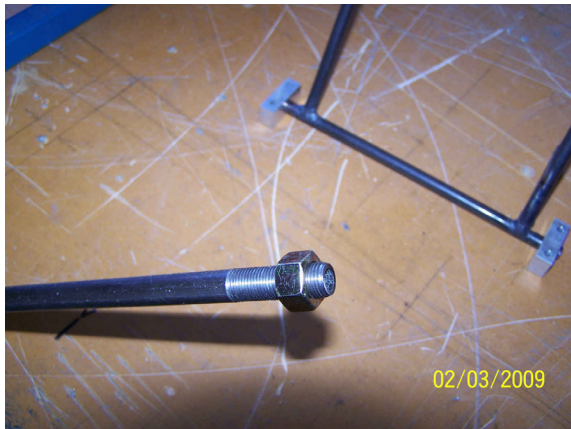
Upper rod, with thread cut...to be trimmed to length when installed in wing.
